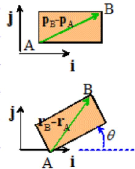
$$\underline{r}_B - \underline{r}_A = R(\underline{r}_B - \underline{r}_A)$$
